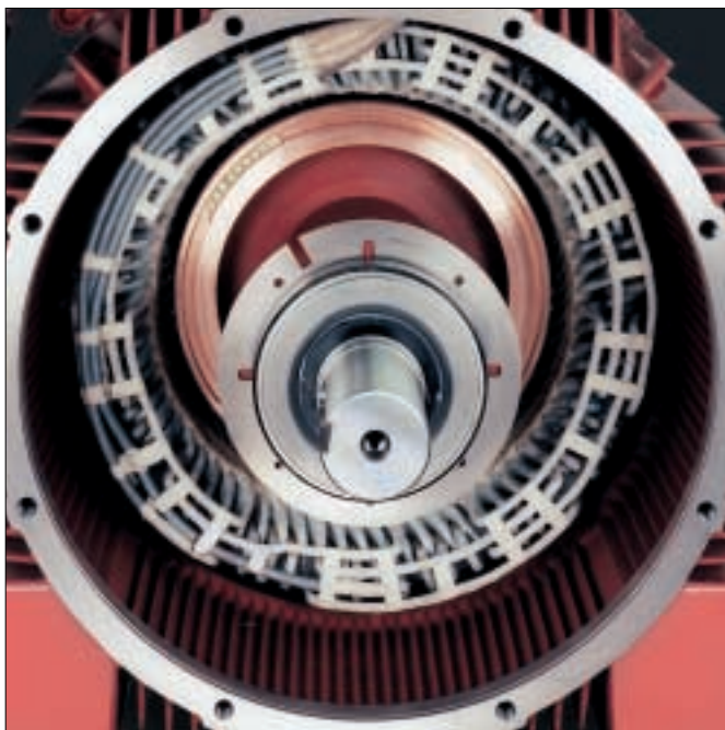
Connecting side of endwinding
