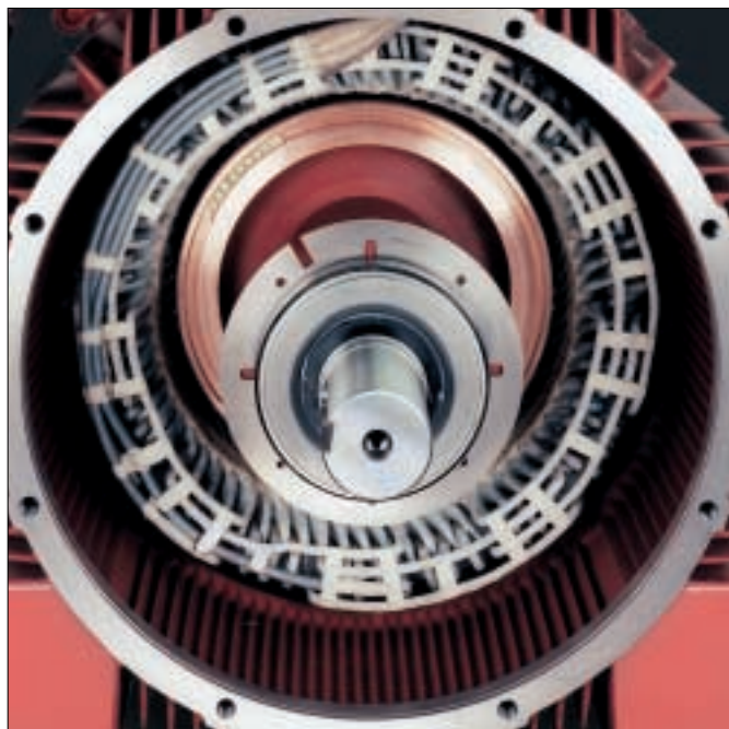
Connecting side of endwinding
