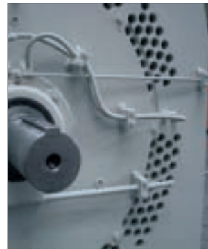
Anti-friction bearing with lubricator and grease drain
