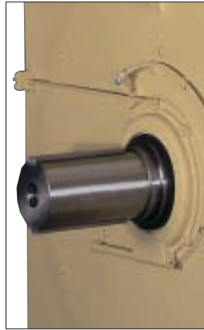
Antifriction bearing with lubricator and grease drain
