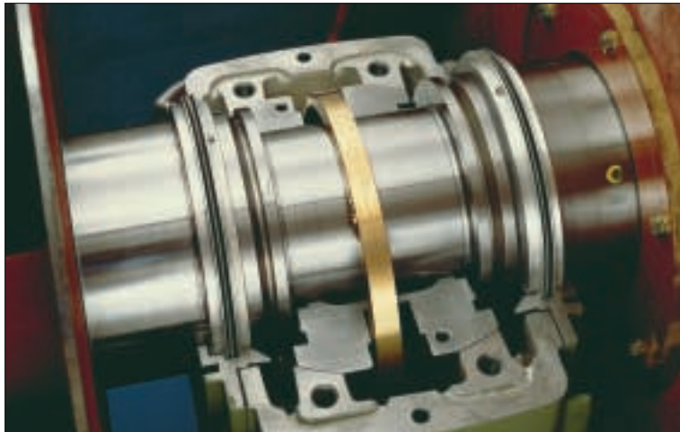
Sleeve bearing with ring oiler
