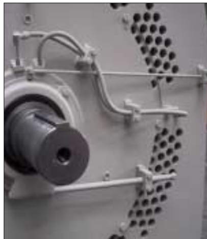
Antifriction bearing with lubricator and grease drain
