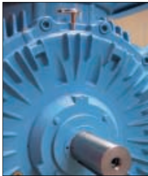
Anti-friction bearing with lubricator
