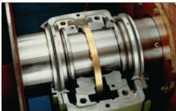
Sleeve bearing with ring oiler
