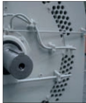
Anti-friction bearing with lubricator and grease drain
