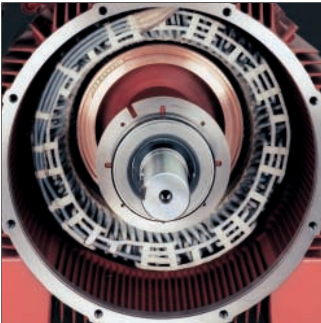
Connecting side of endwinding
