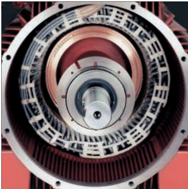
Connecting side of endwinding
