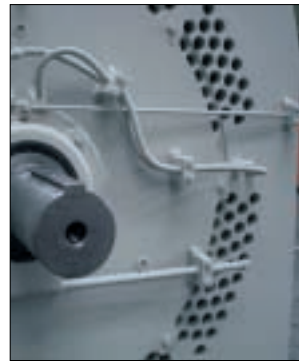
Anti-friction bearing with lubricator and grease drain
