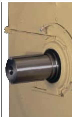
Antifriction bearing with lubricator and grease drain
