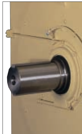
Antifriction bearing with lubricator and grease drain
