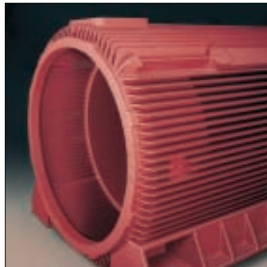
Casting of a size 560 frame
