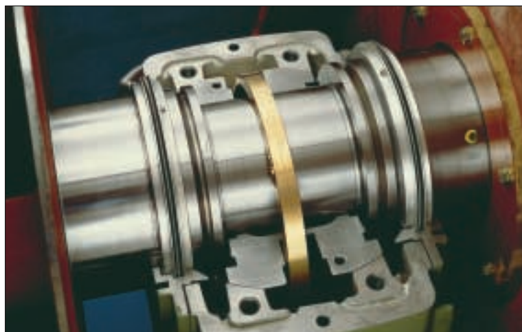
Sleeve bearing with ring oiler
