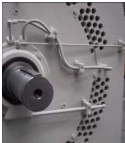
Antifriction bearing with lubricator and grease drain
